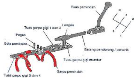
Gambar 3.17. Sistem pengoperasian langsung ( Direct control )
